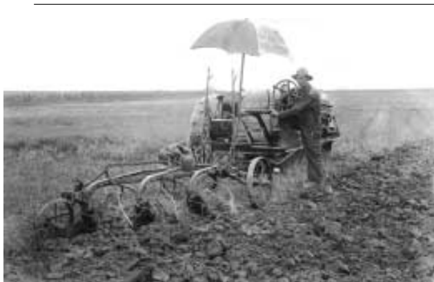
Fall plowing with a 3-bottom plow with comfort seat and umbrella.
