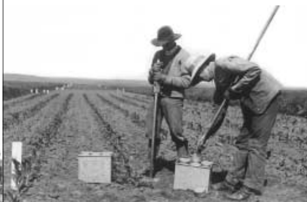
Determining the quantity of soil water using a core sampler that was pounded into the soil, then jacked out; a very time consuming process.
