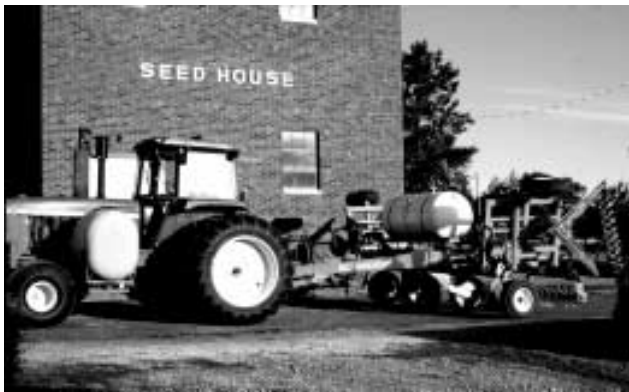
Liquid side tanks on the tractor and anhydrous tank on the V-blade tillage tool allow a dual application of nitrogen and phosphorus fertilizer through tubes on the underneath side of each V-blade.
